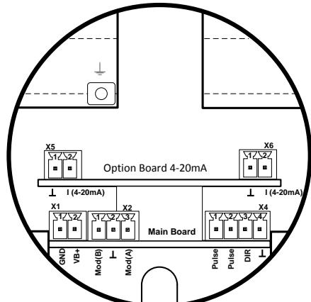
Version with option board 2x analogue outputs galvanically isolated
