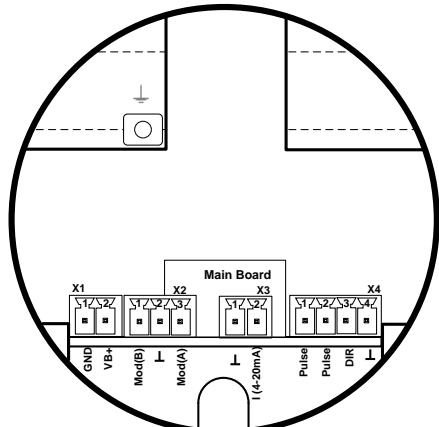
Standard version with 1x analogue output (not galvanically isolated)
