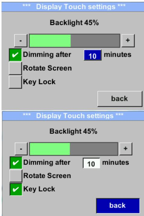
With the button „-“ and with button „+“ it is possible to adjust the backlight / display brightness. The actual / adjusted backlight brightness is showed in the graph „**Backlight**.“
