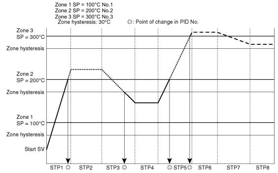
When above diagram shows SV as: Below 200°C → Action with PID No. 1 200°C ~ 300°C → Action with PID No. 2 Above 300°C → Action with PID No. 3
