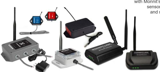
Monnit Mine is designed to work with Monnit's diverse set of wireless sensor types, wireless control and robust, reliable wireless gateways (available in commercial and industrial platforms).
