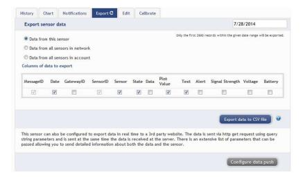
To export sensor data you must first select the date range for the data you want to export. Once the date range is selected, determine whether you want sensor data from the selected sensor only, from all sensors in the network or all sensors assigned to the account. When you are finished, click on "Export Data" at the bottom of this window. The data will be exported to a comma separated value (.csv) file format. Note: Only the first 2,500 records within the selected date range will be exported.
