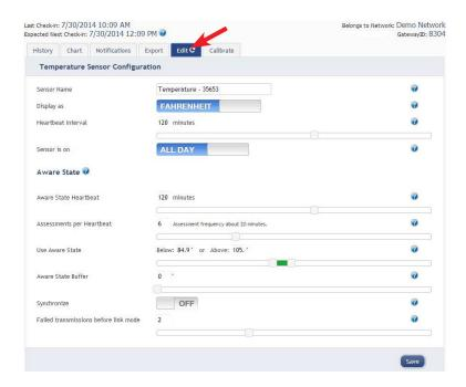
The sensor edit panel allows you to set the primary configurations for the sensor. Mousing over the question mark icon by each setting will provide an explanation of that setting. When you have finished making changes, press the "Save" button at the bottom of this section.
