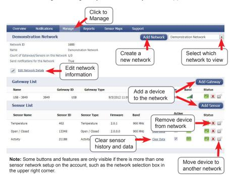
If more than one sensor network is setup on the account, you can easily move gateways and sensors from one network to another by clicking on the "Move Device" button at the far right of the device's "Status" section.
