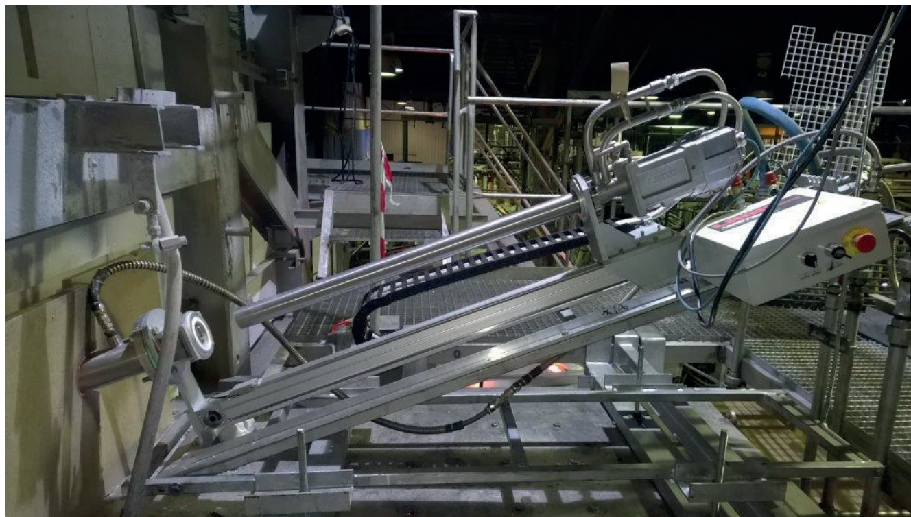
NIR-B Glass retracted from the glass melt tank
