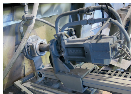
NIR-B Glass inserted through melt tank wall
