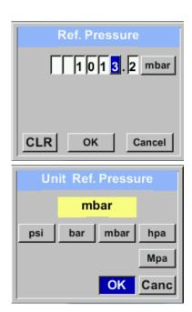
In order to change, e.g. the unit, first select by pressing key ,, $\triangle$  " the field "*Units*" and then key "OK".
