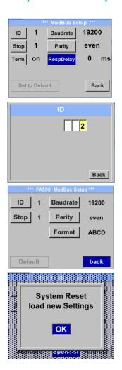
For changes, e.g. the sensor ID, first select by pressing key " $\Delta$ " the field "ID" and then key "OK".
