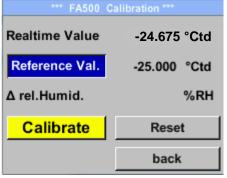
Here, a one-point calibration can be performed
