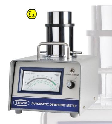
The Model SADP is fully self contained and comes complete and ready for use with batteries installed, Calibration Certificate traceable to National & International Humidity Standards, two metres of PTFE sampling hose, instruction manual and a specially designed heavy duty leather case with shoulder strap.
