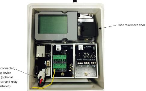
Battery disconnected; no charging device plugged in (optional analog sensor and relay modules installed)
