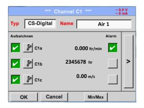
After defining the *name* and confirmation with *OK*, the sensor configuration is completed.
