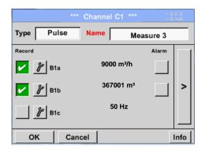
Typically the value with unit of **1 Pulse** is standing on the sensor and can directly entered to the **1 Pulse** = description field.
