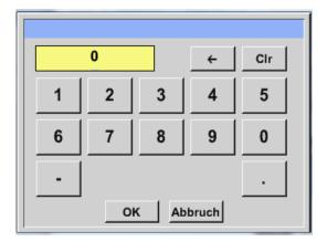
Pressing the button *const. Value* requests the input of the *const. Value* into the text field.
