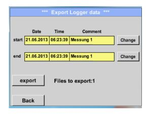
Use the *Change* buttons to adjust a period between *start* and *end*. Stored measurement data in this period are exported
