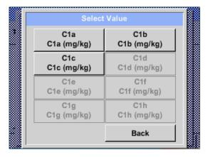
Pressing the respective channel button e.g. *C1b* will select the measurement channel
