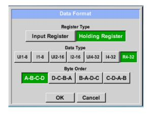
With the buttons *Input Register* and *Holding Register* the corresponding Modbusregister type will be selected.
