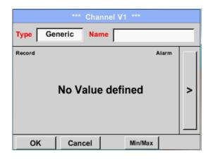
By pushing the Text field *Name* a Sensor name could be inserted.
