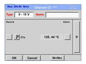
Please see the scale of the sensor (here for example Type  $\bf 0$  -  $\bf 10V$  corresponds to 0 - 250 ° C) from the data sheet of the connected sensor.
