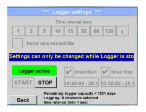
After the start and stop time activation and the created settings, the *Start* button will be pushed and the data logger is armed.
