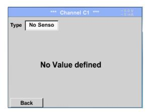
Is used to declare a not currently needed channel as *No Sensor* defined.
