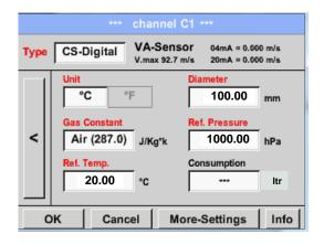
The red labeled description fields indicate, that different values, such as the *Diameter* and the *Type*, have been changed or added.
