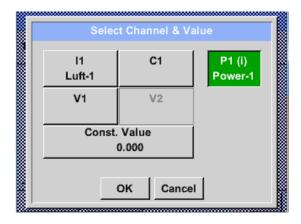
By pressing a button either for HW-, virtual channel or const. Value e.g. *C1* a list of all available measurement channels or measurement values will appear.
