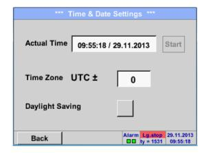
By pushing the *Time Zone* description field and enter the correct *UTC*, you can set the correct time all over the world.
