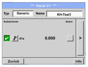
Use the *Record* buttons to select the measurement data that will be stored by **activated data logger**
