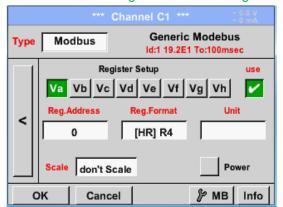
The measurement values are kept in the registers of the sensor and can be addressed via Modbus and read by the DP 510.
