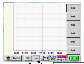
One or more channels for the recording and presentation of measured data can be selected here, such as a dew point sensor or several different sensors.
