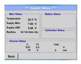
The function System Status offers an overview, fitting voltages and currents on the individual and the entire channel, as well as the power supply of the power supply unit.
