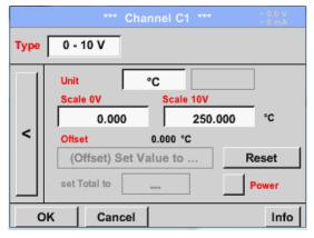
By *Scale 0V* enter the lower and by *Scale10V* the upper scale value
