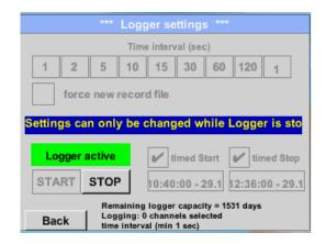
The data logger can be started without activated time settings, use the *Start* and *Stop* buttons for activate and disable. Left below there will be shown how many values are recorded and how long there still can be recorded.
