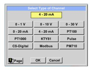
By pushing the button of the required sensor button e.g. 4 -20mA the sensor is selected. Pushing the button **No Sensor** will reset the selection.
