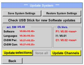
If the DP 500 / DP 510 is correctly connected to USB, and new version available it will displayed.
