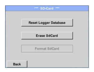
By pressing *Reset Logger Database* all actual stored data on SD-Card will be blocked for use in DS 400. Nevertheless all data are still stored and available for external use only.
