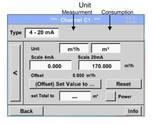
Selection of the units by pushing the text fields for the corresponding measurement and consumption units.
