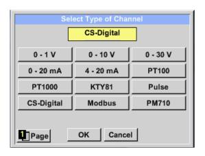
Now the *Type* **CS-Digital** is selected for the VA/FA 400 series and confirmed by pressing the *OK* button.
