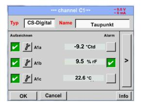
The DP 510 detects, if the connected sensor is a flow or dewpoint sensor of **CS Instruments** and set the CS-Digital subtype automatically correct.
