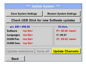
If after pushing the *Check USB Stick for new Software updates* button the following messages in the window appears, then DP 500 DP 510 is not connected properly with the USB stick or no files are available.
