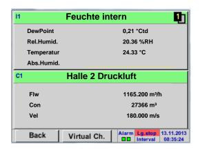
The overview of *Channels* shows the current measured values of all connected sensors.
