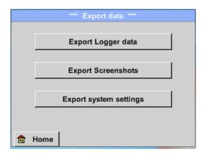
With Export Logger data and Export system settings the recorded measurement data and saved settings can be transferred to a USB stick.
