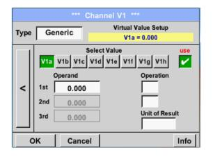
Every virtual value has to activated by selecting the respective *Value-Button* e.g. *V1a* and pushing of the *Use Button*.
