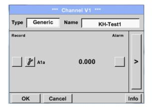
The Resolution of the decimal places, the Short Name and Value Name are found under the **Tool button**
