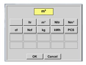
By *Unit Pulse* you can choose between a flow volume or a power consumption unit.
