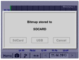
After pressing the Screnshot button a menu (see left) appears where the storage target, USB Stick or internal SD-card, could be selected.
