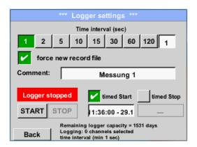
By pushing the *timed Start* button and then the date/time description field below, the date and the start time can be set for a data logger recording.
