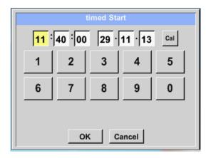
After pushing the *date/time description field* a window will appear where the yellow marked area of the time or date can always be set and changed.
