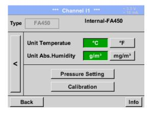
In the upper block it the units for the temperature,  $^{\circ}C$  and  $^{\circ}F$ , as well as for the absolut humidity,  $g/m^3$  and  $mg/m^3$ , can be selected.
