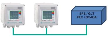
RS 485 network (Modbus RTU) or Ethernet (Modbus/TCP)
