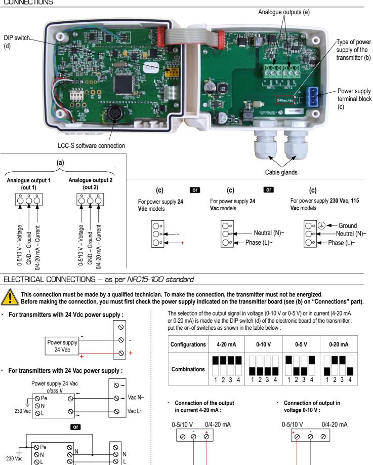
For transmitters with 115 or 230 Vac power ۶ supply:
