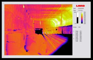
*Temperature Profiles inside the furnace*
