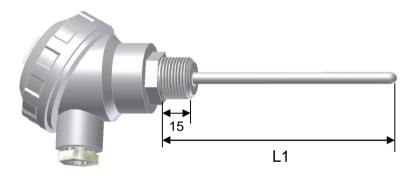
Large Alloy Head, Ceramic 3 way block, PT100 Class A, 6.4mm OD 316 Stainless Steel stem. Max Temp 260°C. 1/2" BSPT Standard.
