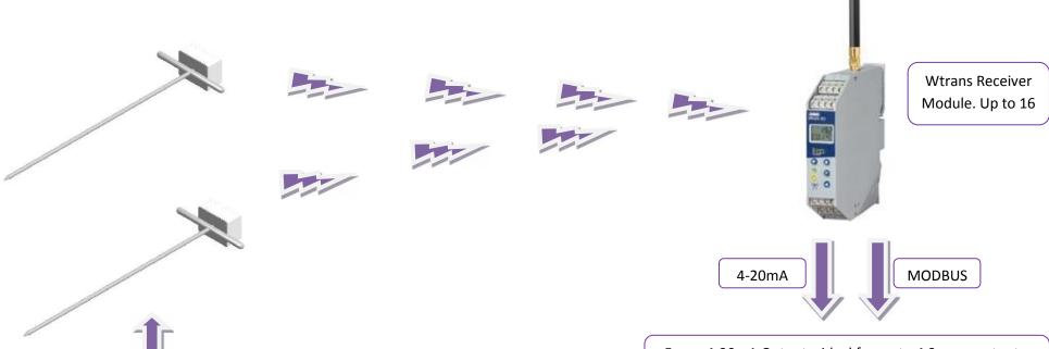
**Wireless Compost Temperature** T-Bar Stab Probes **Battery Powered** 2 Meters
