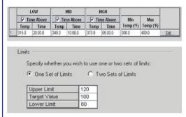
Select the analysis function used in the SPC operation (e.g., Datapaq Value) then input the parameters for that analysis. The analysis function is applied to each profile in the SPC list and reported on the SPC chart.
