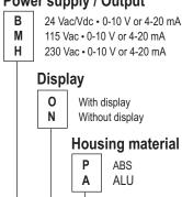
$\begin{tabular}{ll} \textbf{Example: CP302-BOA} = pressure transmitter type CP 300, with measuring range of $-500/+500$ Pa, with power supply $24$ Vac/Vdc, 0-10 V or 4-20 mA output, $-200/+200 mA outpu$ with display and alu housing.
