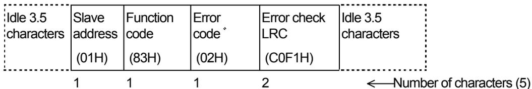
In a response message during normal operation, "1" is set to the MSB of the function code (83H). An error code 02H (non-existent data address) is returned as the response message for the error content.
