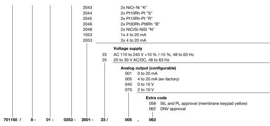
1. The first number on the measuring input means single probe "1" or double probe "2"
