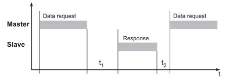
t1Waiting period 1, consisting of 3.5 character transmission times, plus the time that the slave (sensor) requires for processing the data requestt2Waiting period 2 that the master has to observe before it starts a new data request:
