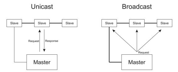
The master controls data exchange by cyclically requesting the slaves in the overall bus. The slaves (e.g. JUMO tecLine sensors) only have a response function. The master has write and read access to the slaves. This enables data to be communicated between master and slave devices in real time. Slaves cannot communicate with one another directly. In order to transfer data from slave to slave, the master must extract data from one slave and then transfer it to the next.
