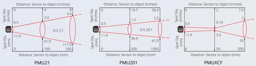
Diagrams show the diameter of the measured spot versus the distance from the lens of the sensor. The measured spot sizes shown here contain 90% of the energy the sensor detects. We normally recommend the target size should be at least twice the measured spot size for maximum accuracy. All PyroMiniUSB models will measure at longer distances than the diagrams show, with a larger measured spot size.
