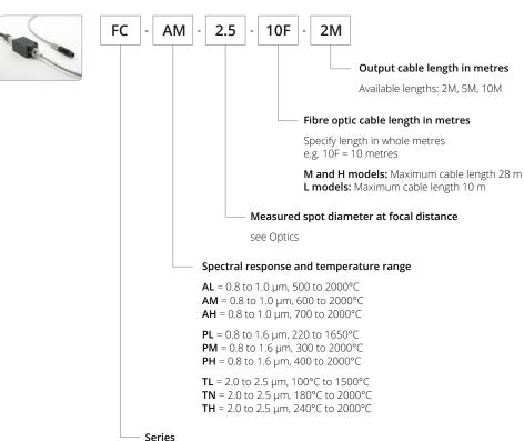
**FC** = FibreCube fibre optic infrared temperature sensor
