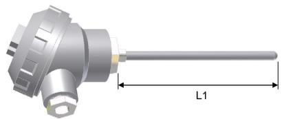
Small Alloy Head, Ceramic 3 way block, PT100 Class A, 6.4mm OD 316 Stainless Steel stem. Max Temp 260°C.
