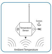
Monnit Wireless Temperature Sensors monitor the ambient temperature around the sensor. The sensors feature mounting flanges and can be attached to most surfaces using the included mounting screws or double-sided tape.
