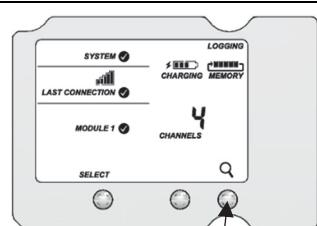
Press the Search button. The magnifying glass icon will blink while the station is in search mode waiting for sensor nodes to join the network.
