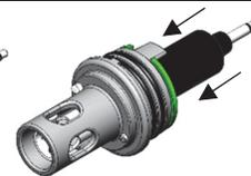
Wipe the outer plastic body of the electrode dry with a soft cloth or paper towel (never touch the glass bulb). *Gently and slowly* push the electrode into the new end cap. Gently twist it so the holes in the sensor align with the holes in the end cap.
