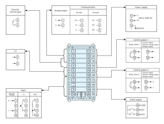
Crimp-type terminals fit M3.5 screws.
