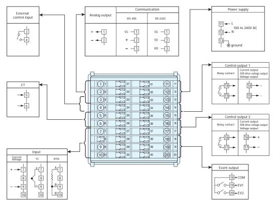
Crimp-type terminals fit M3.5 screws.
