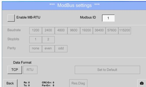
By communication via Modbus TCP the **Modbus Id** have to be set only and confirmed by pressing **Apply** button.
