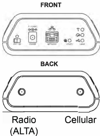
Connect the antennas to the back of the gateway as seen in the diagram.
