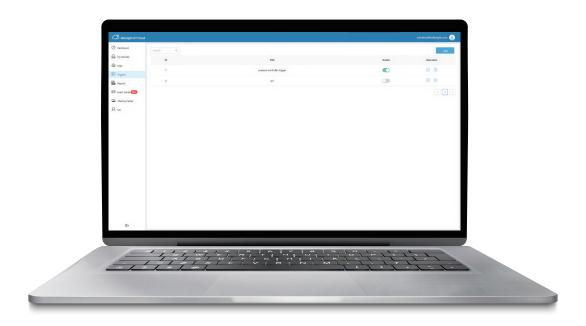
The Trigger interface allows users to customize multiple combinations of conditions and triggers. Based on the processed data, Milesight IoT Cloud provides users with many options of trigger warnings, thus adding preventive monitoring for users.
