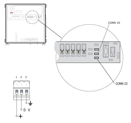
current loop connections are electrically isolated
