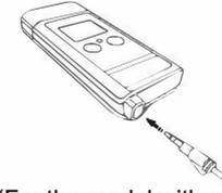
(For the model with external temperature probe, please make sure the sensor is completely inserted into the device.)
