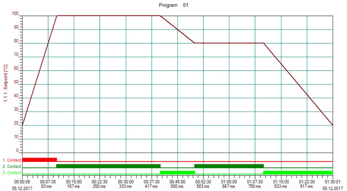
The setpoint value programmed in a section (e.g. 20 in section 1) changes gradually during that section to the setpoint value of the next section (e.g. 100 in section 2). This produces a course in a ramp shape. For a setpoint value to remain constant in a section (e.g. 100 in section 2), the same setpoint value must be specified for the next section (e.g. 100 in section 3).
