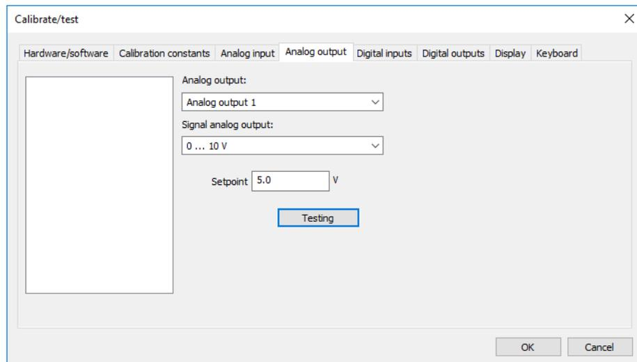
After selecting the corresponding signal type and entering the setpoint value, the corresponding value is output at the analog output by pressing the "Test" button. The output value must be measured and entered in the "Measured value" field. Finally, the setpoint value and actual value (measured value) are displayed for comparison.
