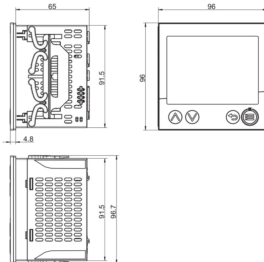
Panel cut-out according to DIN IEC 61554
