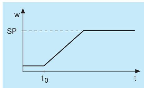
A tolerance band can be set around the setpoint value curve to monitor the actual value. If the actual value deviates from the tolerance band, the tolerance band signal is activated.
