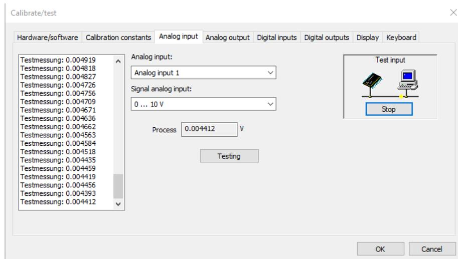
After selecting the corresponding signal type and pressing the "Test" button, the value at the analog input is continuously measured and displayed in the "Act. value" (last value) field as well as in the display field (left; all measured values). The continuous measurement is terminated by pressing "Stop".
