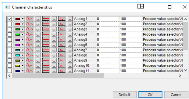
Up to 18 channels in a line chart (channels can be individually hidden) can be shown in the visualization. The X axis depicts the time course of the signals in the diagram. The values of the signals are represented on the Y-axis, whereby only one signal can ever be selected for the main y axis. The values of the other signals are represented either on additional Y axes (auxiliary y axis) or without a y axis.
