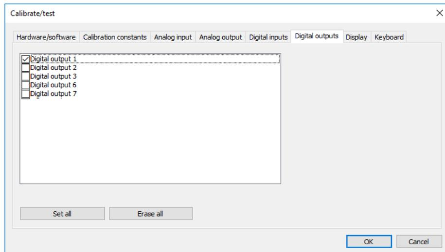
Set all: All outputs are set to TRUE after the button is pressed (checkmark in checkbox).
