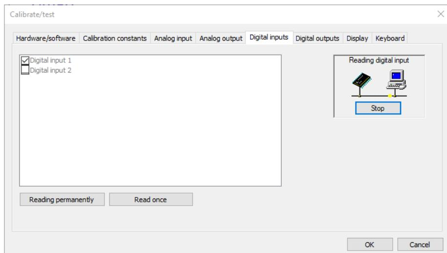
Read permanently: After pressing the button, the inputs are continuously read and the display is continuously updated. Reading must be ended using the "Stop" button.
