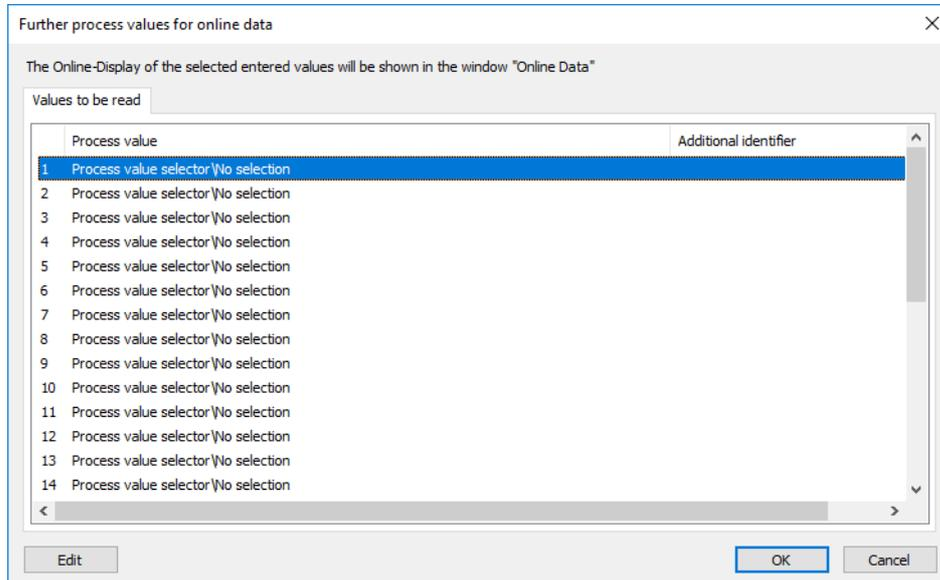
After pressing the "Edit" button (or double clicking on the relevant line), the process value for the previously marked line can be selected:
