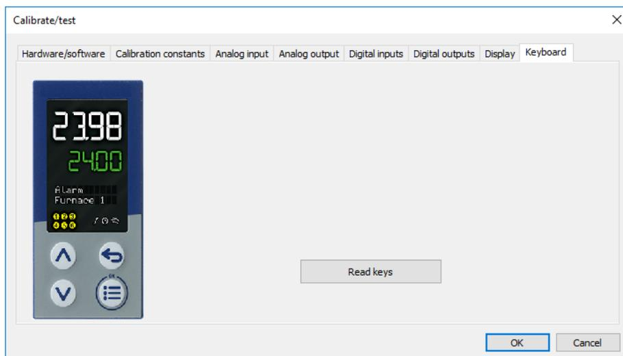
After pressing the "Read buttons", each press of a button on the device is shown by a red circle around the corresponding button of the device shown here:
