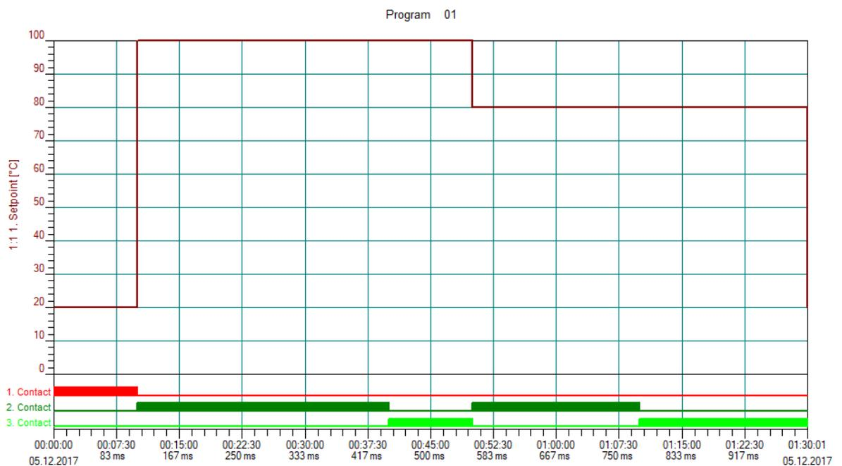
The setpoint value programmed in a section (e.g. 20 in section 1) remains constant for the entire duration of this section. At the start of the next section, the setpoint value jumps to the value for this section (e.g. 100 in section 2).
