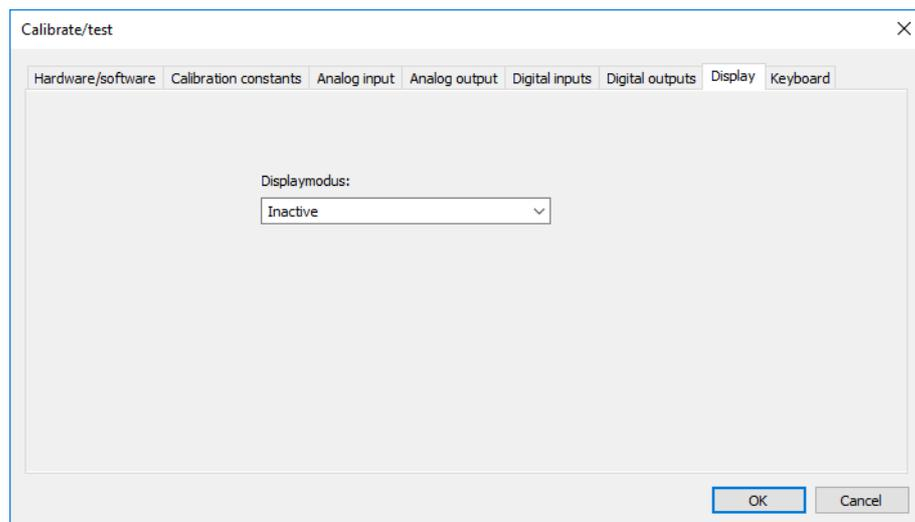
Inactive: The function is not active. The display corresponds to the standard display in calibration/testing mode.
