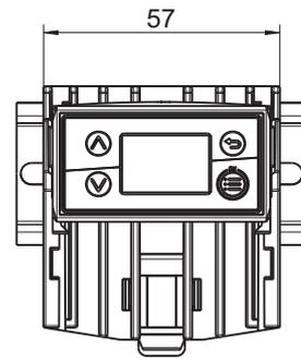
Type 702111 (format 116) mounted on DIN rail (see accessories)
