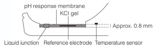
● **Sectional drawing of tip of Flat sensor.**
