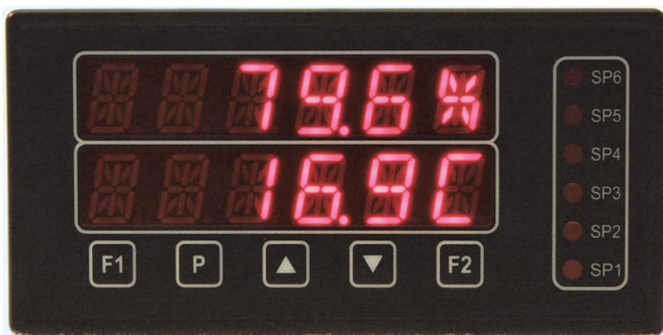
**SP(X)** The setpoint LED's are used to indicate active setpoints.
