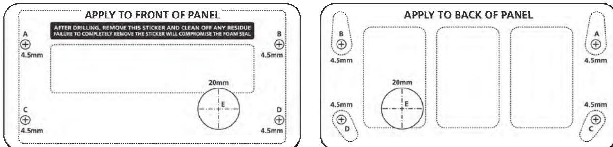
This unit is supplied with two stickers to assist with installation. Apply the front sticker if you are drilling from the front of the panel, and back sticker if you are drilling from the back of the panel.
