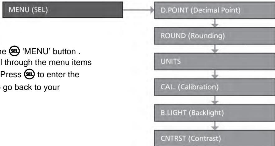
From the operational display area, press the 'MENU' button . 'D.POINT' will appear on the display. Scroll through the menu items using the 'UP' and 'Down' buttons . Press to enter the selected menu, or the 'BACK' button to go back to your operational display.
