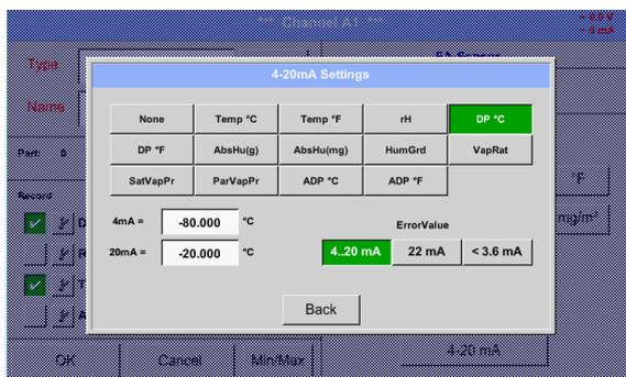
This menu allows the adjustment / assignment of the measurement value and the scaling of the analogue output.
