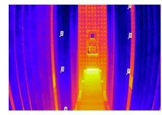
Figure 2. Thermal View inside and Reformer Tube Furnace with data points. Source: <u>AMETEK Land</u>
