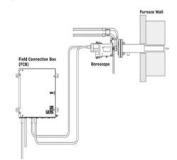
Figure 1. The Thermal imaging cameras are inserted into the reformer, with the end of the imager  $\frac{1}{4}$ " from the inside reformer wall refractory. Imagers are water and air-cooled, ensuring accuracy in the hot atmosphere of the reformer. Source: AMETEK Land
