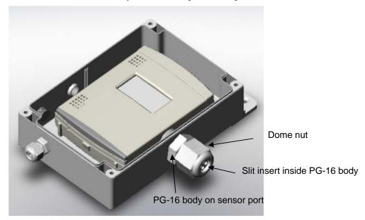
5. A slit insert is located inside the PG-16 body. Push the slit insert out from the inside of case. It is easier to do this if you lift the logger out of the case. You may need to push the slit insert out using a pen (capped end), pencil (eraser end), or other blunt instrument.
