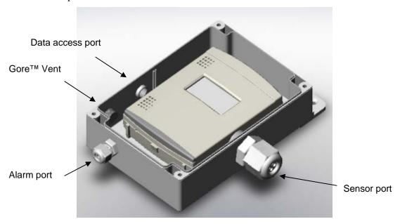
4. Remove the dome nut from the PG-16 body in the sensor port on the protective case.
