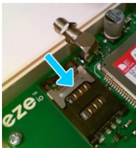
Slide the metal latch down to release hinged lid.
