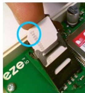
Insert SIM card into the lid. Orient cut corner top left.
