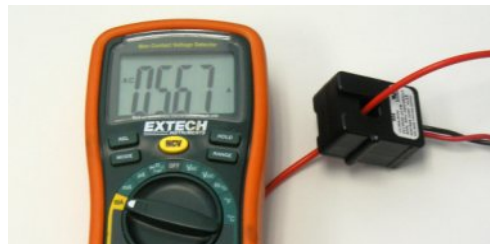
Current sensor and reference meter, 5.67A
