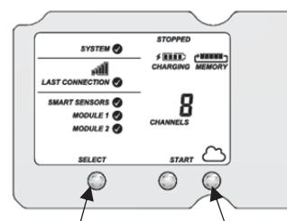
Press the Select button to return to the main LCD screen
