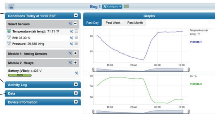
View graphs of sensor data (if enabled); hover over a series to see individual data points on the graph
