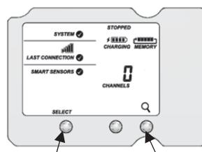
Press the Select button to view the smart sensor channels
