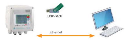
The measured data stored in the data logger integrated in DS 400 can be read-out via USB stick.
