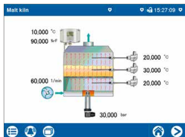
Visualizing a plant: process screen of a malt drying kiln with integrated measured value display
