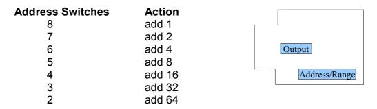
Channel 2 has switch 8 on (start at 1 then add 1), switches 2 to 7 are off.
