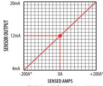
\*Field Adjustable from  $\pm 200$  to  $\pm 200A$  (not applicable to customer-specified factory scaled models)
