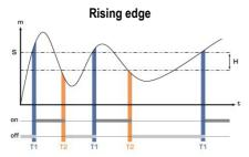
Measurement (m) > Threshold (S) during the time-delay  $T1 \rightarrow Alarm$  activation.
