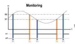
The alarm goes off when the measurement is outside the low and high thresholds.
