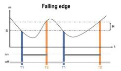
Measurement (m) < Threshold (S) during the time-delayT1  $\rightarrow$  Alarm activation
