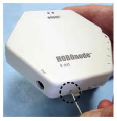
**LED Indication**: While the node is searching for a receiver, the **RED** and **GREEN** LEDs will alternate blinking.
